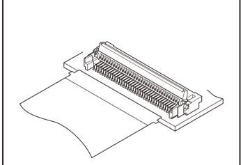
A substantial size for the 0.3mm pitch connector ensures easy handling. Moreover, since this connector accepts a FPC with protrusion providing secure as well as foolproof mating at the customers production line.
