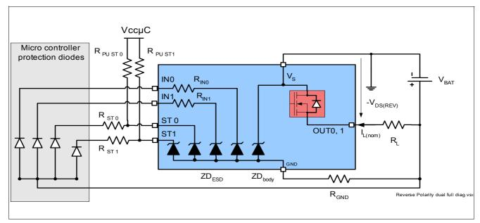
Figure 10 Reverse polarity protection with external components
