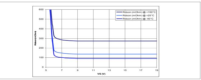
Figure 4 Typical ON-State Resistance
