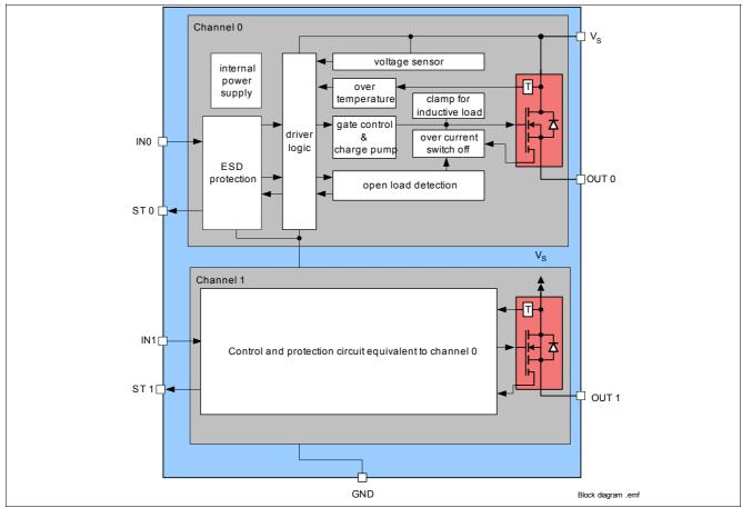
Figure 1 Block diagram for the BTS4160DGA
