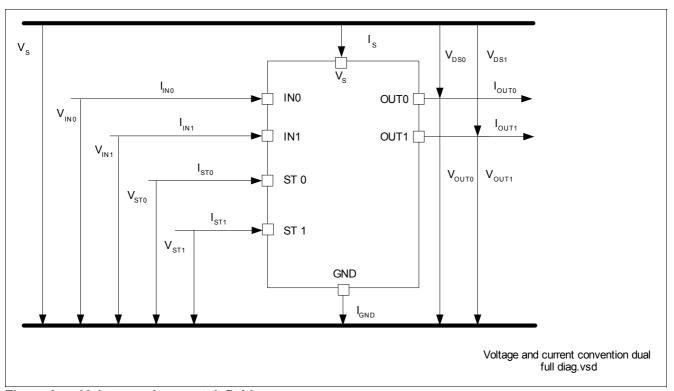
Figure 3 Voltage and current definition
