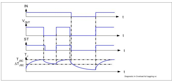
Figure 15 Sense signal in overtemperature condition
