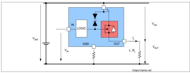
Figure 6 Output clamp (OUT0 and OUT1)
