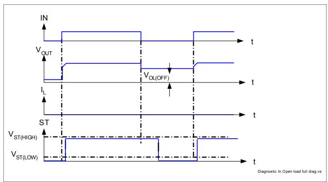
Figure 14 ST 0/1 in open load condition
