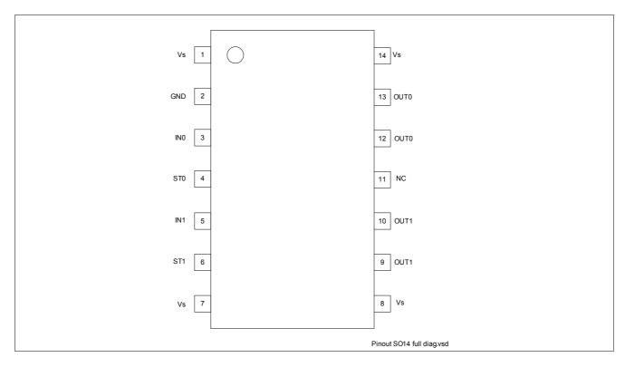
Figure 2 Pin Configuration
