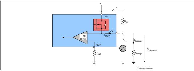
Figure 13 Open load detection in OFF electrical equivalent circuit
