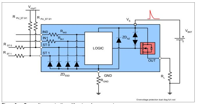
Figure 9 Over voltage protection with external components
