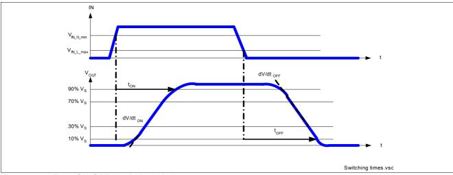
Figure 5 Turn ON/OFF (resistive) timing
