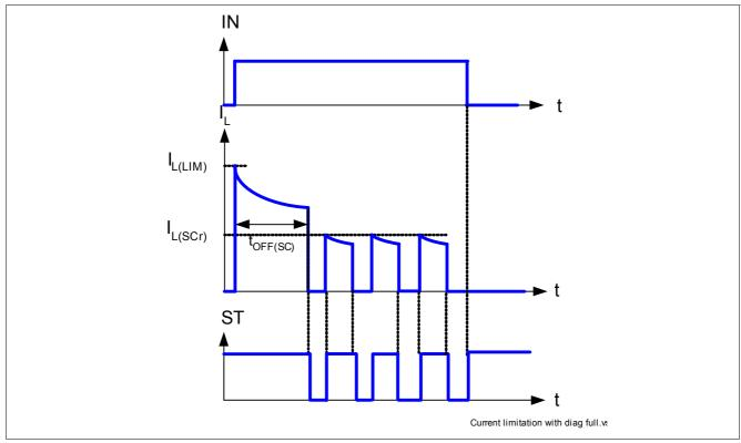
Figure 11 Current limitation function of the time
