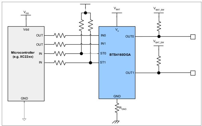
Figure 17 Application diagram with BTS4160DGA
