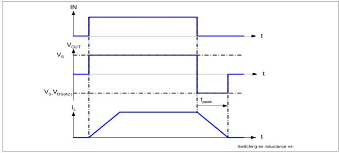
Figure 7 Switching an inductance
