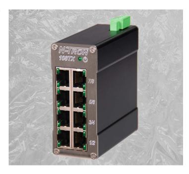
The 108TX-HV supports up to 2,000 MAC addresses, enabling these products to support extremely sophisticated and complex network architectures.
