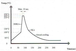
Recommendable wave soldering condition is as follows:
