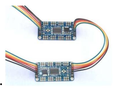
Multiple boards can be chained to control hundreds of LEDs. Using an Arduino, you will run out of memory long before you exceed the chaining capacity of these boards!
