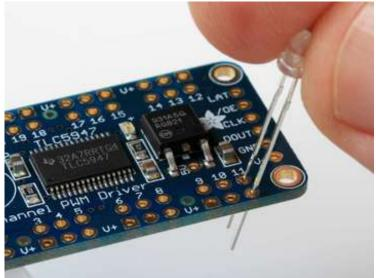
Note that one leg of the led is longer than the other. This is the Anode and should be connected to the V+ hole in the board.
