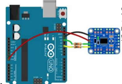
Connect V+ to 4-17V and keep VCC disconnected. Then use 10K resistors or a level shifter between the clock and data wires going into the *first* of the TLC59711
