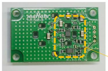
Amplifier and comparator circuits on evaluation board amplifies sensor's output signal and generate digital High/Low signal. (Next page)
